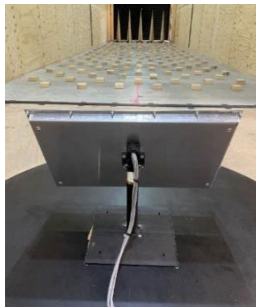
1:6 scale wind tunnel heliostat model
